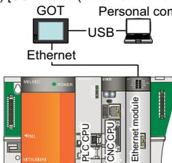
(8) [USB - GOT(Ethernet - PLC CPU module)]
