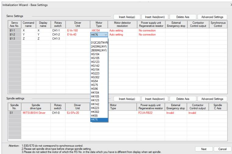
For an existing axis, the settings other than the "axis command name", "axis display name", and "rotary switch" are not displayed on the screen.
