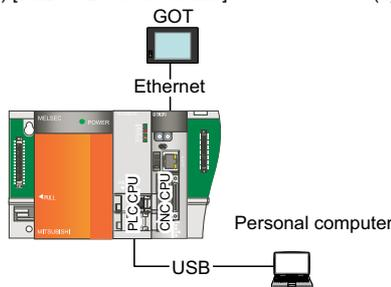
(6) [USB - GOT(Ethernet - CNC CPU module)]
