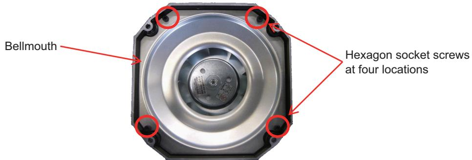
Cooling fan unit (before the bellmouth is removed)
