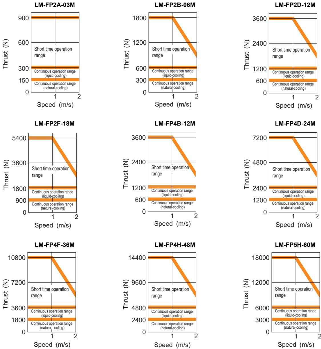
(Note) The above graphs show the data when applied the input voltage of 200VAC(400VAC for FP5H). When the input voltage is 200VAC(400VAC for FP5H) or less, the short time operation range is limited.
