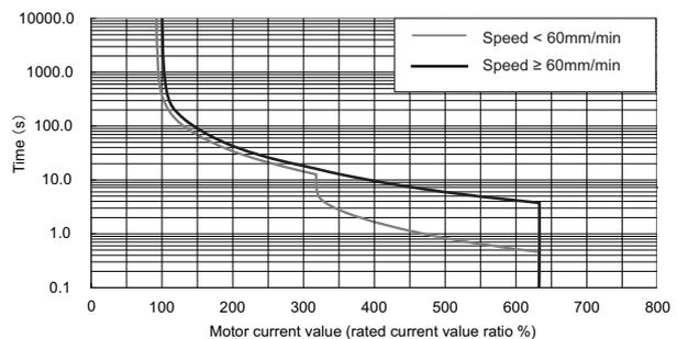
(Note) The characteristics are the same when driving two motors with one unit.
