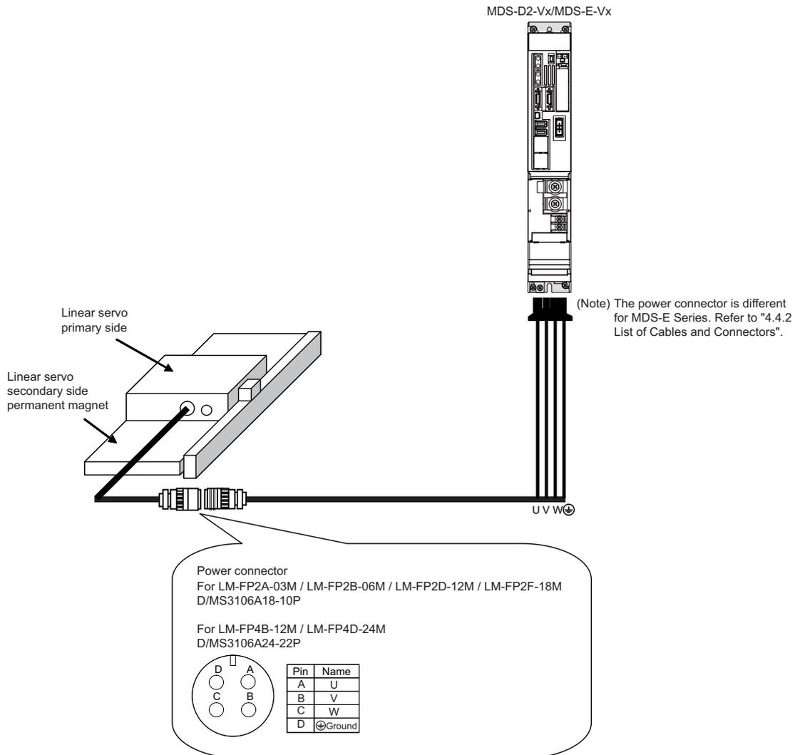
(2) < When the power supply output of the servo drive unit is a terminal type >
