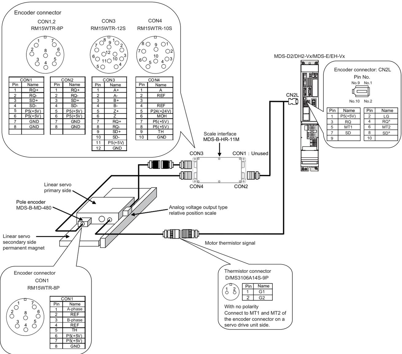
(3) Standard relative position system (When using MDS-EX-HR)
