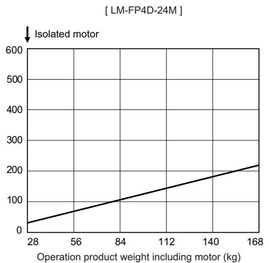
(Note) When driving two motors with one unit, set the standard VGN1 for the operation product weight of one motor.
