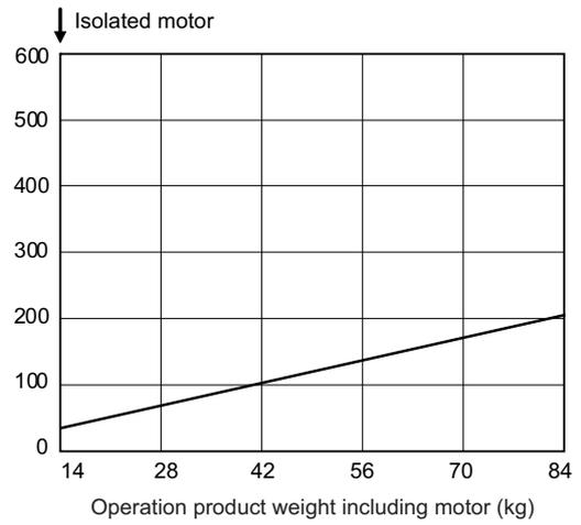
(Note) When driving two motors with one unit, set the standard VGN1 for the operation product weight of one motor.
