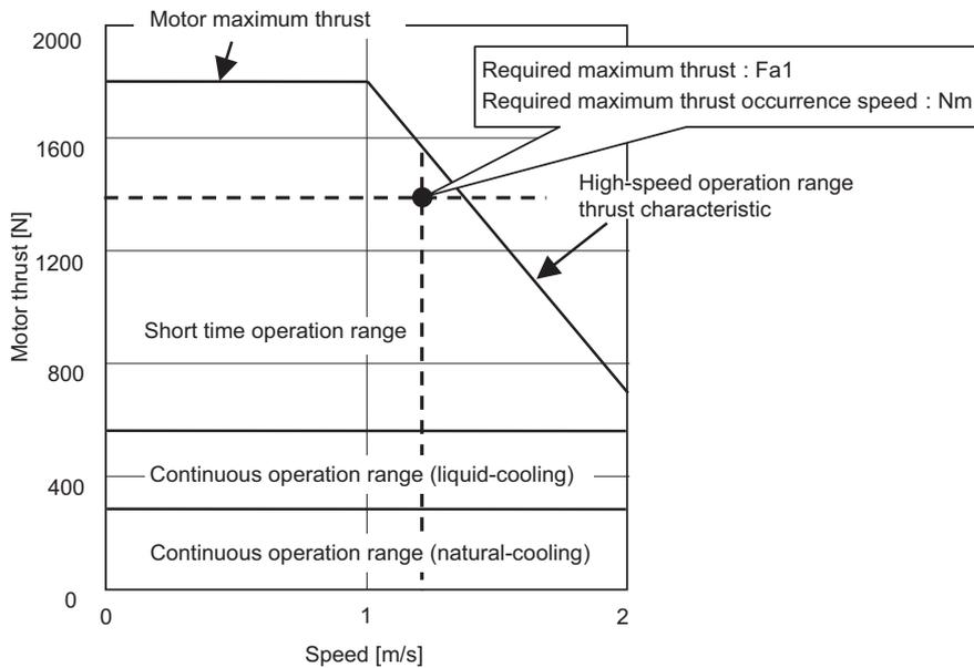
**Motor thrust characteristics**
