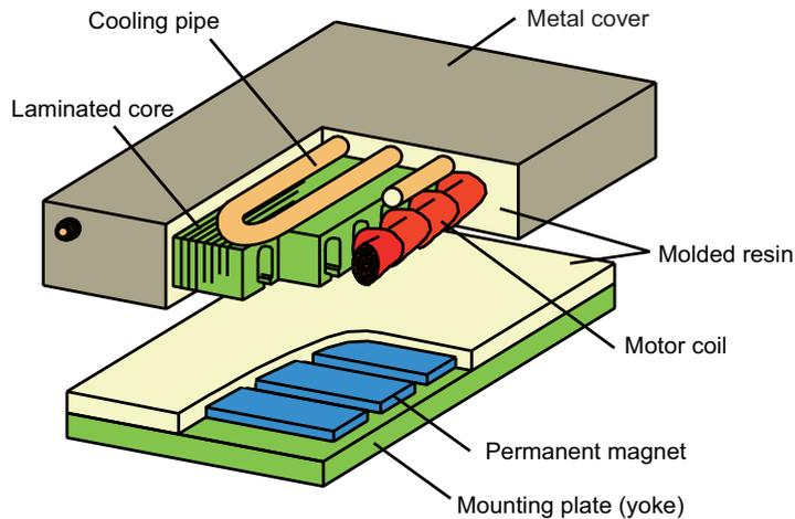
**Fig. 1 Structure of linear servo motor**
