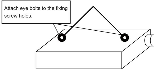
We recommend that you attach the primary side (coil) to the slider and then attach the hanging tools to the slider before suspending the primary side.
