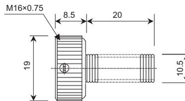
**Servo drive unit connector for CN2/CN3**
