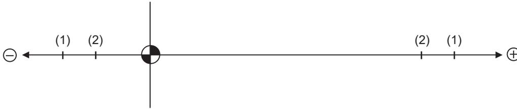
When stroke end is set, the axis will move the distance required to decelerate and stop after the limit switch is activated.
