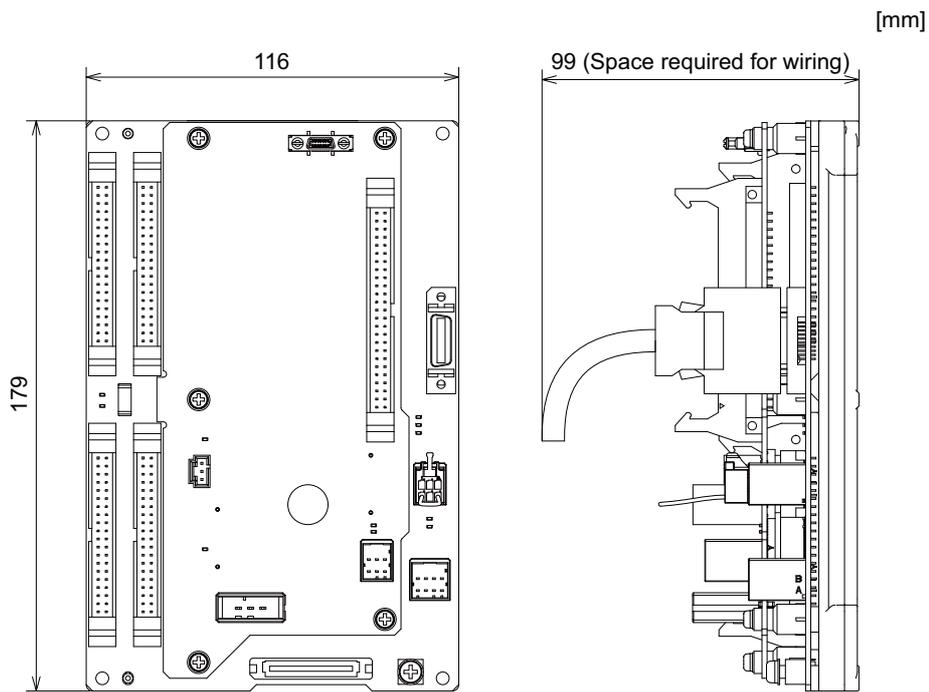
Installation dimension: FCU8-DX731/FCU8-DX750/FCU8-DX760/FCU8-DX761/FCU8-DX834
