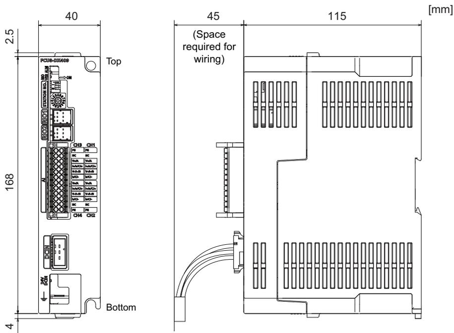
**Installation dimensions: FCU8-DX220/FCU8-DX230/FCU8-DX231/FCU8-DX202/FCU8-DX213/
