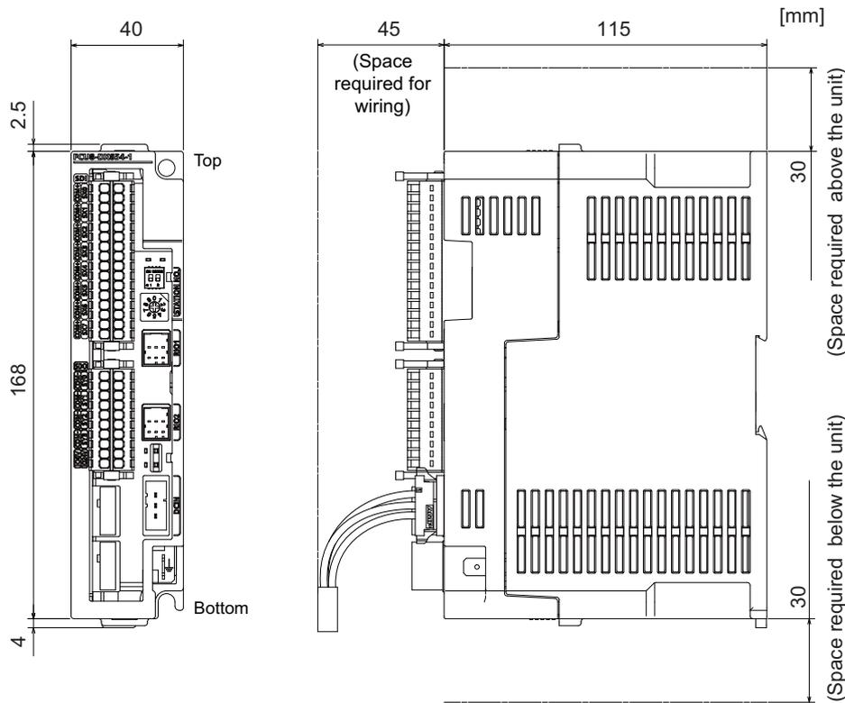
**Installation dimensions: FCU8-DX220/FCU8-DX230/FCU8-DX231/FCU8-DX202/FCU8-DX213/
